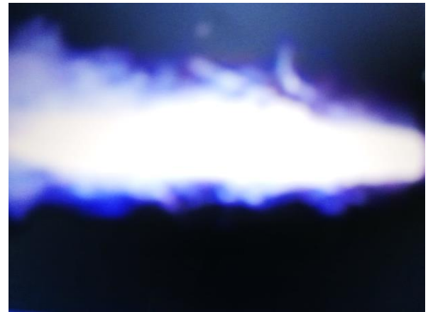
Figure 3. Image of the flame appearance corresponding to the nominal thermal regime
